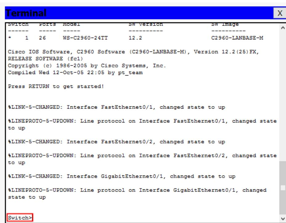
The screenshot shows a terminal window titled "Terminal". It displays the boot process of a Cisco C2960 switch. The output includes:
